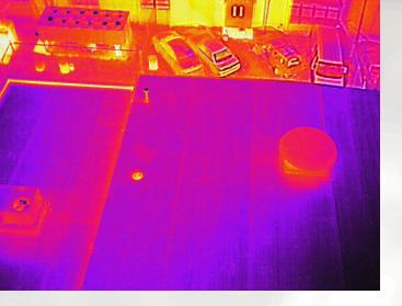
Aerial infrared flat/low slope roof moisture inspections are a non-invasive & non-destructive method of detecting and identifying moisture below the surface of the roof. It is safer in that it does not require ladders and lifts, or "boots on the roof". Aerial infrared roof inspections are more efficient as they do not interfere or disrupt the operation or occupancy of the building & are faster and less expensive than traditional roof inspection methods.
